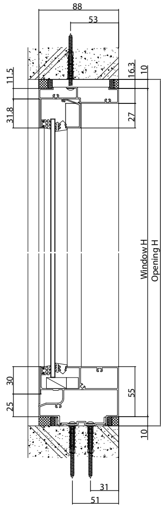
Vertical section: Single fixed window
